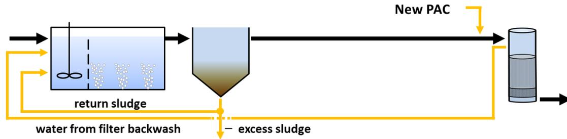
*Separate PAC contact reactor ("Ulmer process")*
